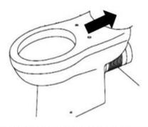
2.Ensure that the toilet pan is level and fully backed against the wall, then mark onthe outer edge of the pan (at both sides), align with each fixing hole located in theside wall of the toilet pan.
